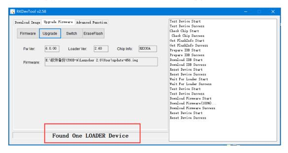
7. When the rooting finished, there will be "Reset Device Success" reminder on the right side of tool. (Please wait the device to restart and keep USB cable connection during this time)
