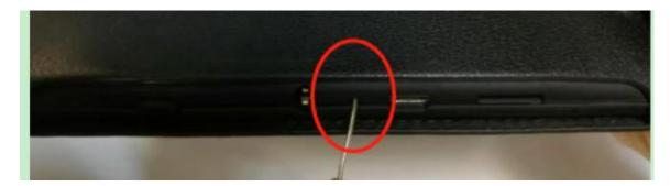
6. After the flash tool reads the device, it will display the "Loader" device. You can only loose the "upgrade key" holding now. Then click "Upgrade" to root the device.
